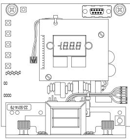
The DCM-3 with Feedback display has been calibrated at the factory and should not require any further adjustments.
