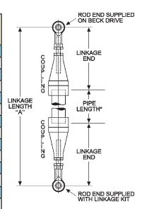
\*NOTE: To calculate length of pipe required, subtract "Length of 2 Linkage Ends" (shown in table above) from Linkage Length "A" (shown in diagram above).
