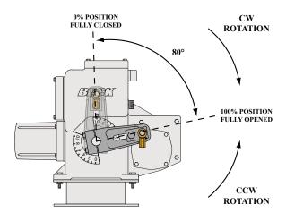
NOTE: The crank arm in the figure above may be adjusted to any start angle. The orientation and rotation shown here has been randomly selected for the purpose of this example.
