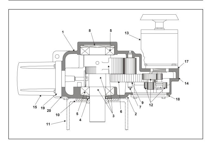
TYPICAL ACTUATOR COMPONENTS FOR MODELS 11-409 / -469\*
