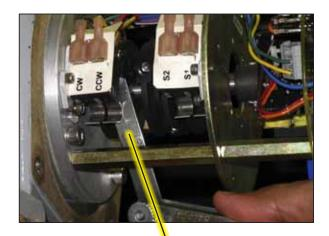
.030" (.75 MM) SHIM SHOULD BE INSERTED BETWEEN ALL LEVERS AND CAMS WHEN SETTING SWITCHES.
