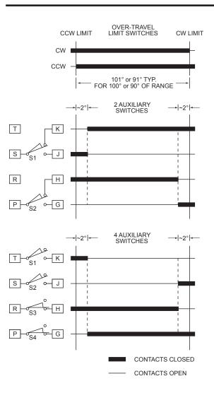
STANDARD OVER-TRAVEL LIMIT AND AUXILIARY SWITCH SETTINGS
