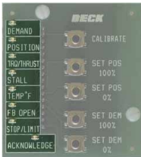
STATUS INDICATION LEDs
