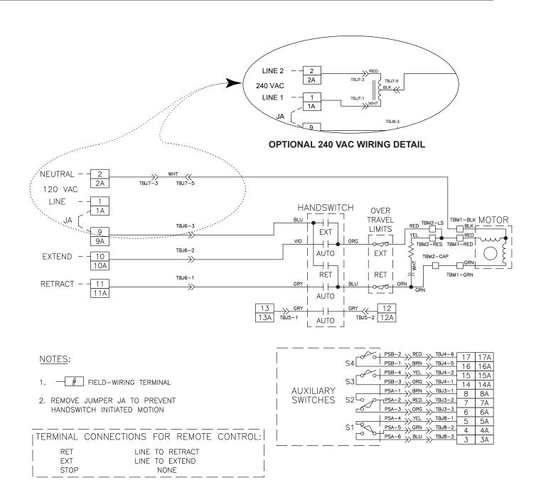
**TYPICAL OPTION 3 WIRING SCHEMATIC**
