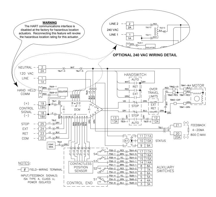
**TYPICAL OPTION 9 WIRING SCHEMATIC**
