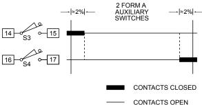
Standard Over-travel Limit and Auxiliary Switch Settings
