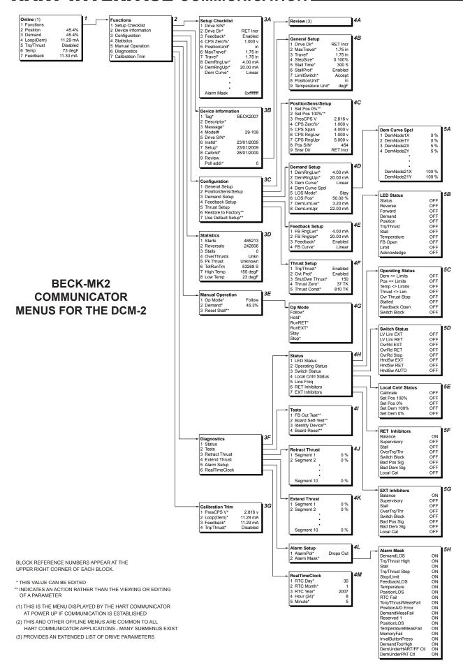
The DCM-2 board is the control center of the drive. Drive configuration and calibration are accessed and set through the DCM-2 board. Using the HART® interface requires a HART® compatible communicator. Typically, a universal model 275/375 HART® communicator is used, but any device, computer or controller capable of communicating with HART® devices and supporting the Beck DCM-2 device description can be used.
