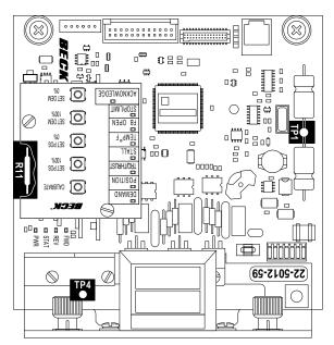
DCM-2 Board showing Resistor R11 and Test Points TP1 & TP4
