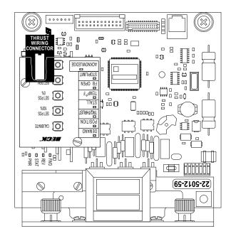
DCM-2 Board showing location of Thrust Wiring Connection
