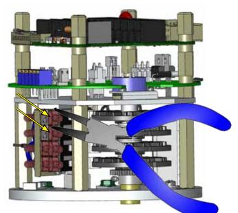
Interchange the limit switch wires (Push on connectors shown without wires for clarity)
