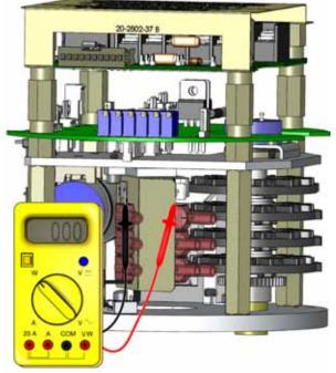
Meter connections for CW switch (Push on connectors shown without wires for clarity)
