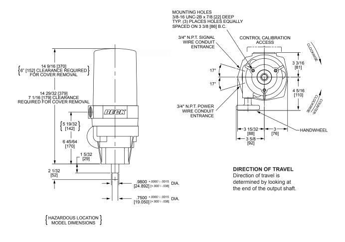
All dimensions are in inches and [mm] unless otherwise specified. Threads and tapped holes are specified as Unified Thread sizes only. Conduit pipe threads per American National Standard Taper Pipe Threads (N.P.T.).
