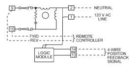
neutral (terminal 2). Customer must supply two wires for analog control: Connect to terminal 11 (-) and to terminal 12 (+). Customer may supply two additional wires to monitor the analog position feedback signal: Connect to terminal 13 (-) and to terminal 14 (+). The actuator's feedback circuit power supply is derived from the 120 V ac line, therefore the feedback signal must be wired to a "4-wire" type, non-powered analog input.
