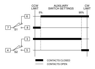
The auxiliary switches are opened and closed by cams that are driven by the actuator output shaft. Setting the switch position involves moving the actuator output shaft to the desired positionthen inserting a small screwdriver into one of the slots on the appropriate cam (see illustration below) and rotating until the cam operates the switch.
