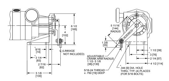
\* Standard dimension shown for mounting bracket, .344 dia. hole thru, typ. 4 places for 5/16 bolts (consult factory if different bolt hole pattern is needed).
