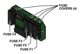
6. When finished replacing the fuse(s), reinstall the Input Fuse PCB and enclosure following this procedure in reverse.
