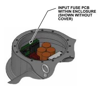
Remove and retain the cap head screw securing the Input Fuse PCB (22-5016-13) to the Input Power PCB (22-5016-12). Remove the Input Fuse PCB by gently pulling it free from the connector.
