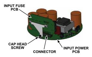
Replace any open fuse. Remove the fuse cover by gently squeezing it on either end and pulling the cover away from the board. Replace the fuses only with the appropriate type (shown on the PCB board).
