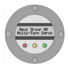
The Red and Green LEDs indicate that the actuator has reached the open or closed position. The position associated with the two LED colors is user configurable through the Close LED setting. However, by default the Green LED indicates a closed condition and the Red LED indicates an open condition. The yellow LED always indicates the actuator is in-between the open and closed positions.
