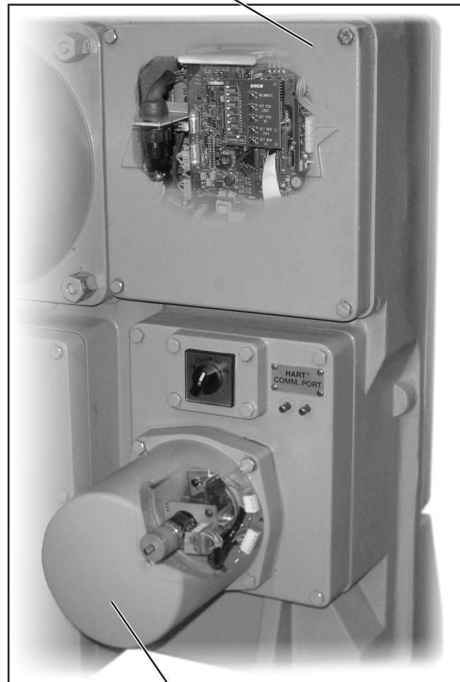
CONTROL END COMPARTMENT
